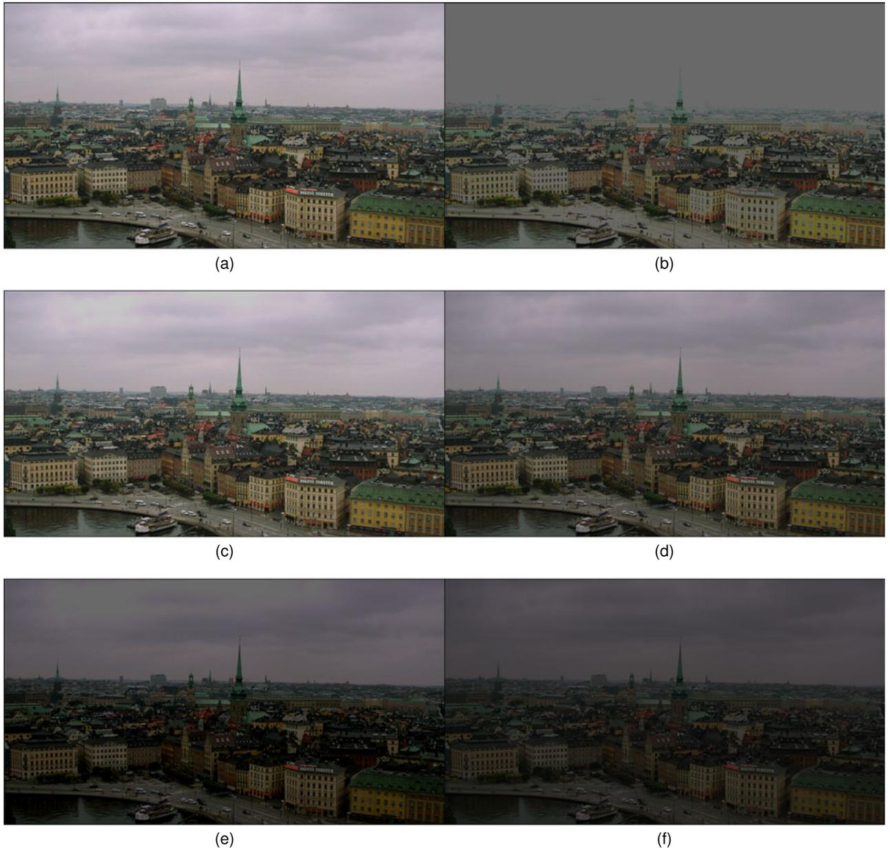
Fig. 7. (a) OldTownCross frame under full backlight,  $B_M$ . (b) Lowest-quality OP without contrast enhancement and 89.9 percent power reduction. (c) Highest-quality OP with 42.8 percent power reduction. (d) Highest-quality OP using [11] and 43.8 percent power reduction. (e) Lowest-quality OP with contrast enhancement and 89.9 percent power reduction. (f) Lowest-quality OP using [11] and 91.2 percent power reduction.
