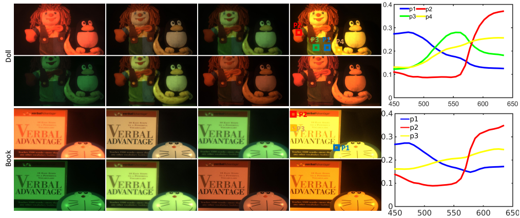
Fig. 11. Real color images captured by our proposed 2 \times 4 camera array system with heterogeneous wideband filters. These two scenes are both captured under indoor iodine-tungsten illumination and we can obtain the illumination spectra through capturing the standard white board. we also randomly select several points with different colors and illustrate their reconstructed 24-channel single-spectral reflectance curves in the rightmost column.
